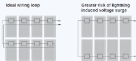
Figure 4: Wire loop design recommendation
